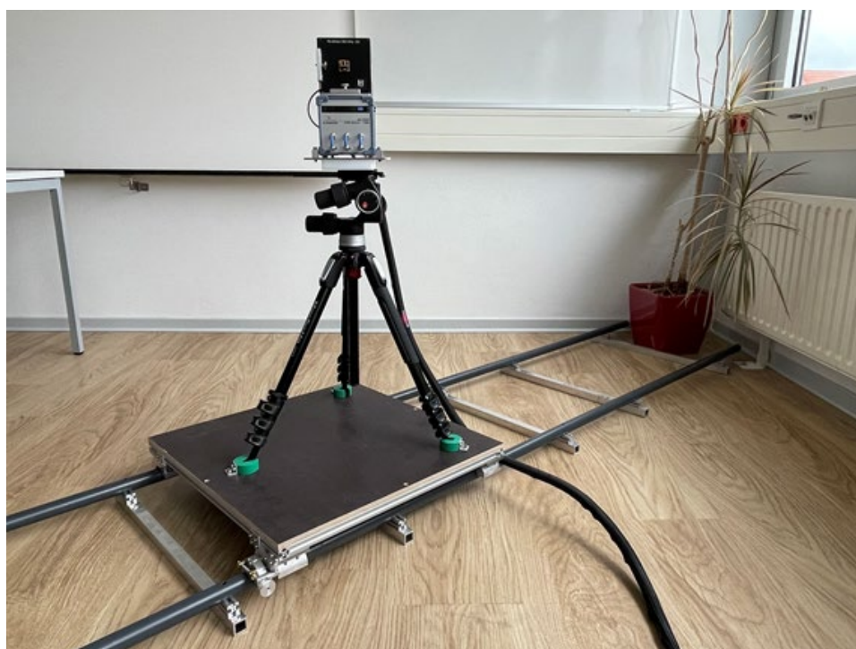
Figure 4 Rail system used for dynamic measurement scenarios
