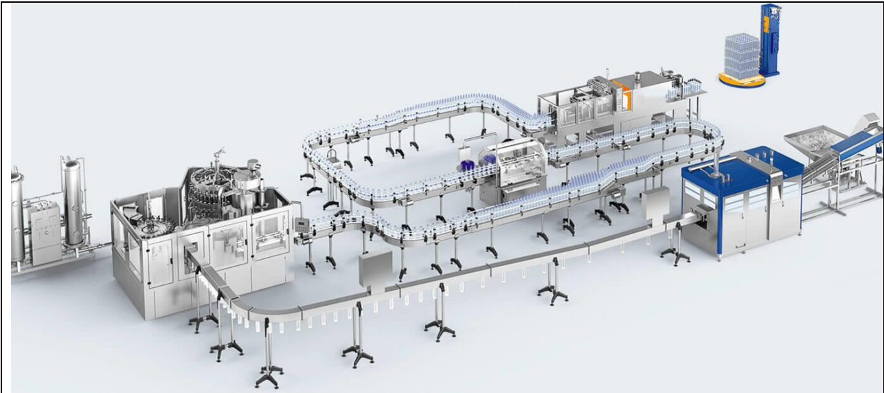
Beverage Production Line. Dimensions: L20m x W10m x H3m
