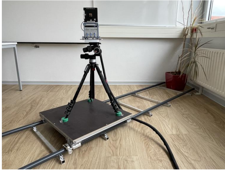
Figure 22 Rail system used for dynamic measurement scenarios
